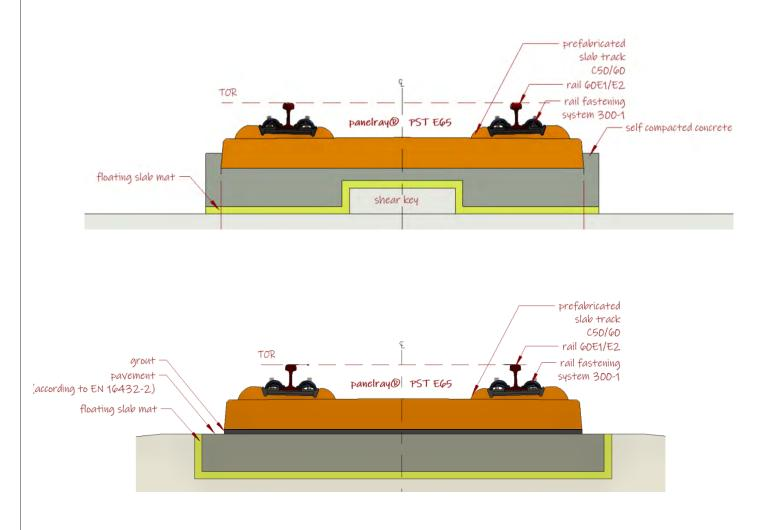
Considering the floating slab mat application concepts, the following graph is given for the vibration mitigation solution of Panelray<sup>®</sup> prefabricated slab track system.
